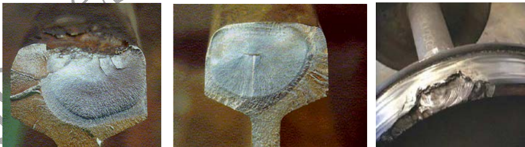
Figure 2 – Examples of progressive crack development in railway component
